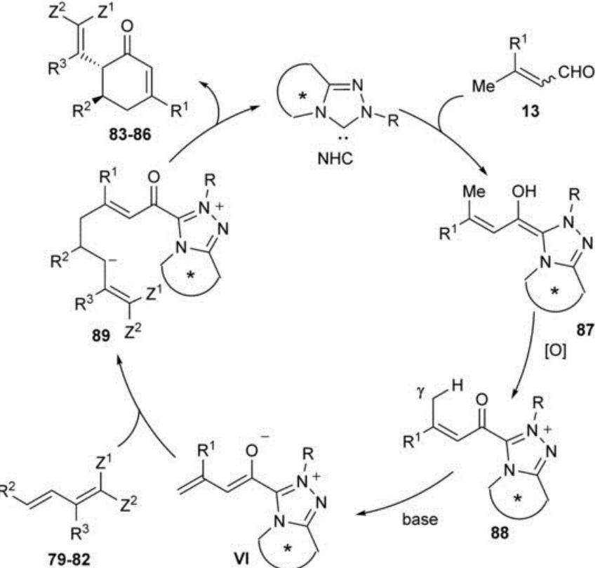
Synthesis of diaryl cyclohexenones via 1,6-addition of azolium dienolates to electron-deficient 2,4-dienes.
